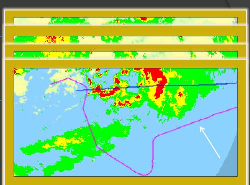
Avoid the storm along the planned path Find another acceptable flight path and gap between convection
