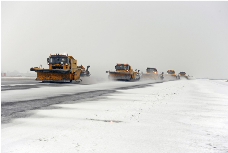
FIG10: A "snow-train", (approximately 13 snow-clearing vehicles, depending on the situations) working on a frozen runway of Paris-CDG.
